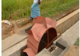
water flow is measured by computerized shutters by canal Automation and water charges are collected accordingly. The canal Automation is very costlier and need so much saftymeasures including yearly maintanence also. But the **Dethridge wheel** is a cheaper water measuring device and with out any yearly maintaince charges and hence, it can be adopted for developing countries like India.
